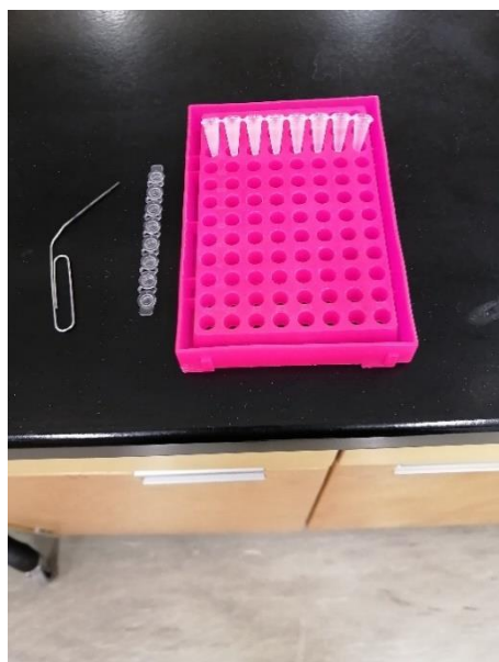
Figure 1: 96 well base with fast reaction tubes, cap strip and paperclip used to poke hole in caps.
